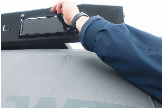
The Off Road Light cover removal tool hooks the upper edge of the cover to remove. -Typical View
