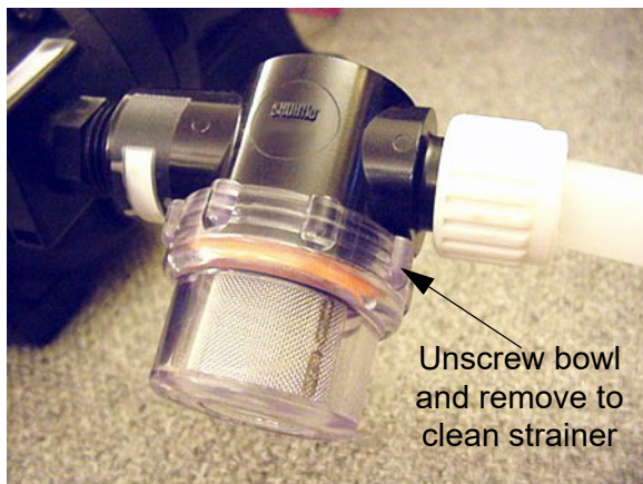
Water Pump Strainer -Typical View
