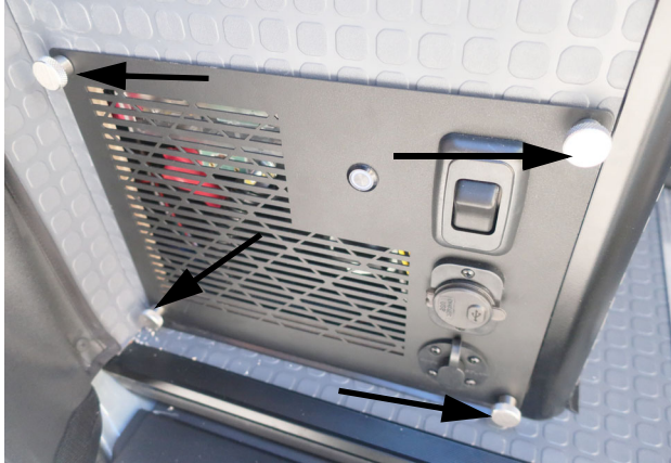
To access the Battery Disconnect Switch, remove 4 twist screws on the panel behind the driver's rear door. -Typical View
