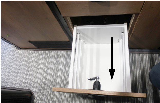
Waste Pump Pull out lower drawer and remove to access. -Typical View
