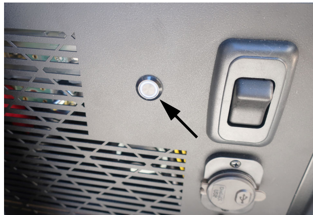
House/Coach Battery Power Controls (Located behind the driver's side rear door). -Typical View
