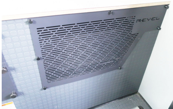
To access the APS Regulator, locate this driver's side rear access panel. -Typical View
