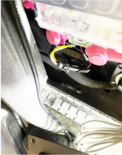
AC Sense and Ignition power connectors connected to enable AC Sense functionality. -Typical View
