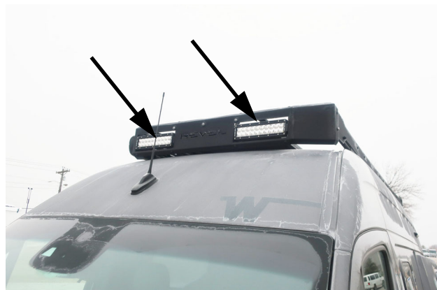
Off Road Lights (Located on the front of the roof rack). -Typical View
