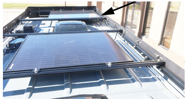
3-Port Solar Cap (Located on the roof) -Typical View
