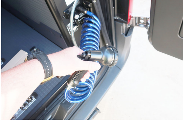
Exterior Shower/Wash Station (located behind rear passenger side door, shown with shower hose hooked up. -Typical View)
